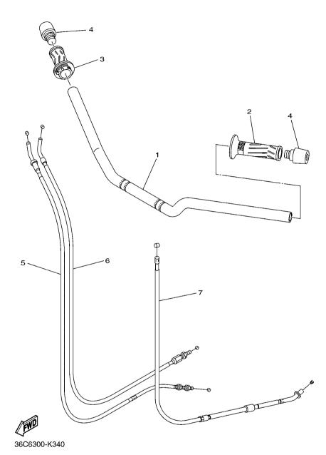
FIG. 33 STEERING HANDLE & CABLE
